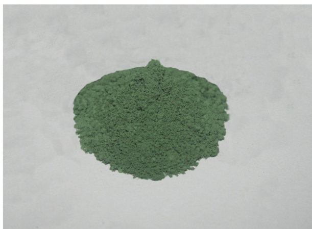
Fig. 1. Original appearance of oxide-based flux powder.
